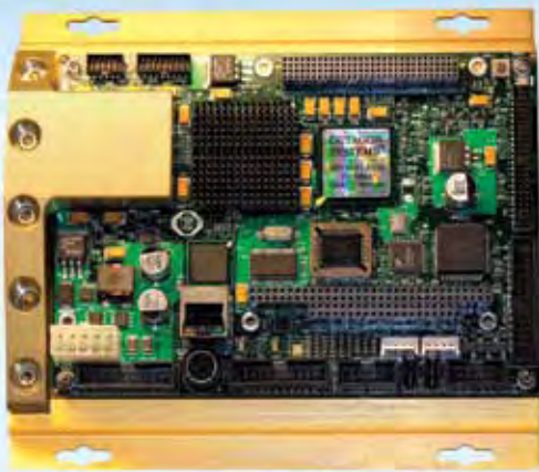
EPIC™ XE-900 CPU, with conductive cooling system
